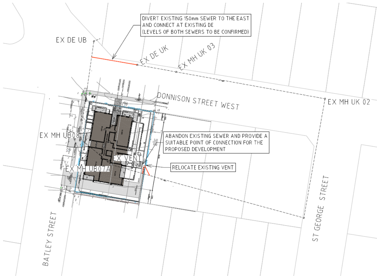
Figure 39 Extract from Wallace Design Group Sewer Main Plans (courtesy of Wallace Design Group )
